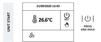
Once the unit is powered and the main-switch is activated, the display turns ON and shows a screen similar to the one you can see above, i.e. unit turned off by KEY.
