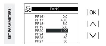
The air flow rate depending on the level of  $CO_2$  in the room. The parameters **PF19** and **PF20** set the min/max PPM limits. Default values are 500/1100 ppm, within which the ventilation varies from min flow rate of 30% to max flow rate of 100%.
