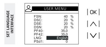
Using the "**UP**" or "**DOWN**" keys, navigate to the LNG parameter and select the value "English" or another language. Confirm the value entered with the "**OK**" key.
