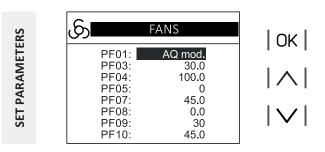
Using the "**UP**" or "**DOWN**" keys, navigate to the **PF01** parameter and select the value "**AQ** mod." Confirm the value entered with the "**OK**" key.
