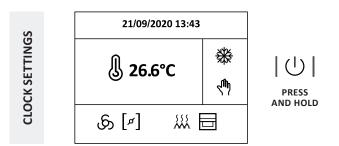
In the event of a prolonged power failure, it may be necessary to reset the unit's RTC clock ("ALARM 29").
