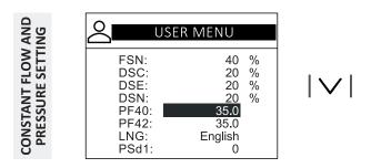
[PLUS Vers.] SET-POINT CONSTANT PRESSURE (Pa x10) [TOP Vers.] SET-POINT CONSTANT FLOW RATE (m<sup>3</sup>/min)
