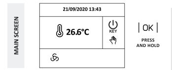
If the unit is ON, switch it OFF. Connect the CO<sub>2</sub> sensor as shown in the circuit diagram. From the main screen, through press and hold of the " $\mathbf{O}\mathbf{K}$ " key, the MENU is accessible.
