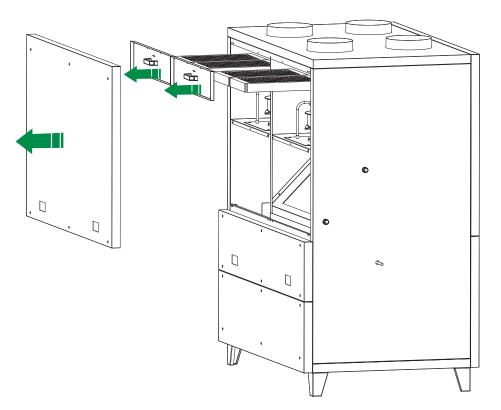
The heat exchanger is not fully removable for this product range, but it can be inspected through the front/rear lower panels of the unit.
