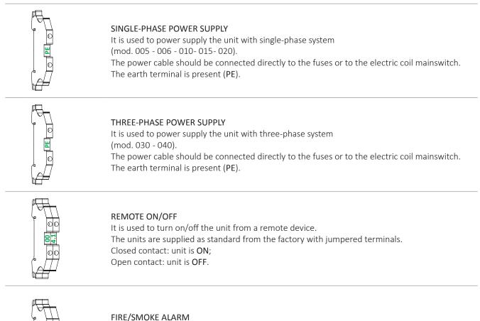
It is used to turn off the unit from an external fire control unit. The units are supplied as standard from the factory with jumpered terminals. Closed contact: no unit alarm works; Open contact: alarm from external fire control unit. The unit stops.
