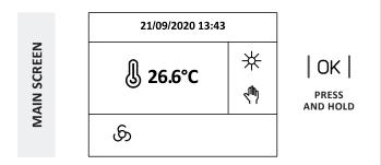
When the unit starts, from this screen it is possible to access to all the menu following explained, through press and hold of the "**OK**" key.
