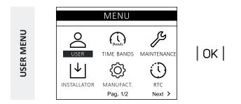
Access to the USER menu does not require a password. In this menu there are all the parameters that the user can freely modify. Press the "OK" key to access.
