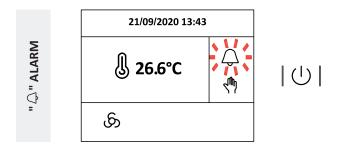
When an alarm is triggered requiring the immediate **STOP** of the unit, the unit automatically turn OFF, the blinking "**BELL**" icon appear on the screen, and the corresponding LED blinks on the left side of the controller.
