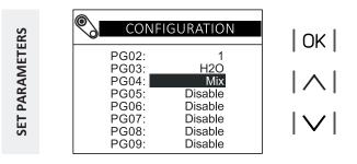
Using the "**UP**" or "**DOWN**" keys, navigate to the PG04 parameter and select the value "Mix". Confirm the value entered with the "**OK**" key.
