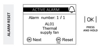
To reset an alarm, is enough to press the "OK" key on it.
