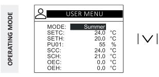
To change the operation mode, use the "**UP**" or "**DOWN**" keys and navigate to the **MODE** parameter.
