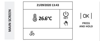
If the unit is ON, switch it OFF. From the main screen, through press and hold of the "**OK**" key, the MENU is accessible.
