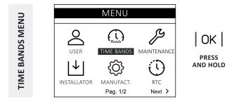
With the unit in operation / switched off, press and hold the "**OK**" key to access to the user menu screen.
