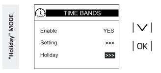
It is possible to set *Unit ON/Unit OFF* mode for a period of absence. This mode is activated from the moment of setting.
